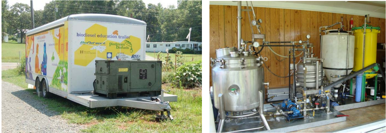
Figure 5: Mobile biodiesel production/education system (Piedmont Biofuels, LLC)
